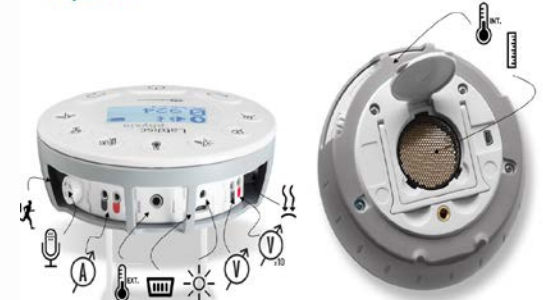
Built-in Sensors Air Pressure, Voltage, Low Voltage, Light, Universal Input, Ambient Temperature, Temperature, Current, Distance, Microphone, Accelerometer, Distance
